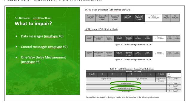
The eCPRI header tells you the message id, so setting up the correct filters in Chimera lets you impair exactly the flow you want to test.
