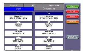
The transmitter and receiver can operate independently, or they can be coupled depending on test setup. Framed signals can be equipped with unstructured or structured payloads with selected test pattern filling the entire test payload (Bulk) or a structured payload (SDH/SONET framed client signal) with or without PDH/DSn multiplexed clients. Layer-based graphical configuration interface allow users to build the test signal in a logical layer by layer sequence
