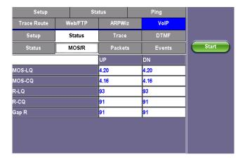
VoIP Call Expert – Emulates an IP phone to place and receive calls using SIP or H.323 protocols. Real-time evaluation of voice quality with a complete set of measurements is available at the end of the call, including packet statistics, jitter statistics, and MOS and R-factor call quality scores. Support VoIP trunk test with bulk call generation of up to 24 simultaneous calls.
