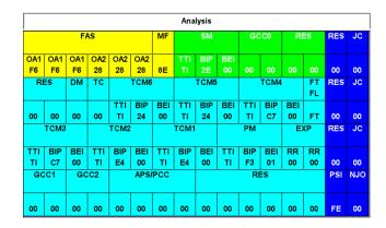
Overhead byte control allows the manipulation and easy encoding of transmitted overhead bytes in both terminated and payload through modes to stress the network responses to various conditions.
