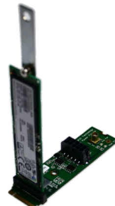
QTL2015 M.2 M-Key Injection Fixture
