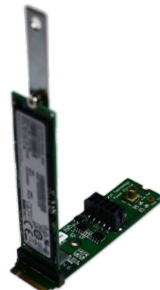
QTL2015 M.2 M-Key Injection Fixture
