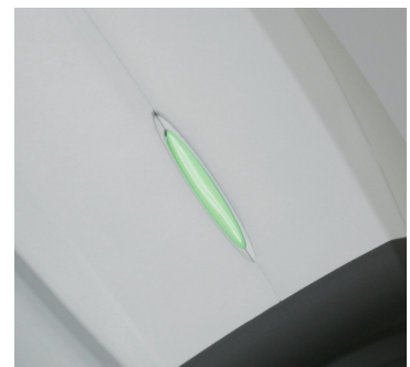
LED irradiator to visualize the discharge (Change the color from red to green upon the discharge)
