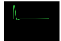
Second order impulse response (damping coefficient 0.7)
