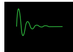
Second order impulse response (damping coefficient 0.2)
